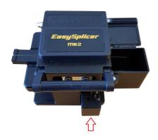
Close the lid of the cleaver and push the sliding part away from you. The fiber will be cut off (cleaved) and get a very straight 90´ angle Lift the fiber holder in order to prevent the fiber from getting dirty.
