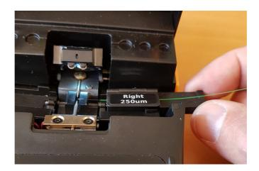
Close the bracket over the v-groove and lock the fibers in position
