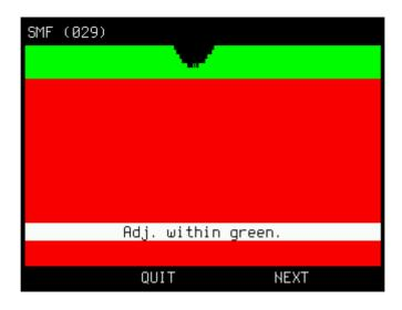
Adjust the upper electrode so that it is within the green area or just outside. But it must not be visible in the red area.
