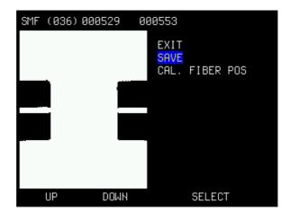
If CAL. FIBER POS Fails and can't position the fibers like in the picture above then Motor position adjustment above needs to be performed.
