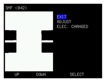
First thing to do is to place a fiber in the v-groove. This will guide the splicer to find the exact vertical center of the fiber.
