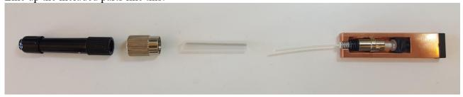
After stripping, cleaning and cleaving of both sides.
