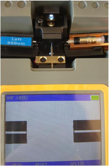
After splicing, open the SOC holder and lift the connector out of the holder. Let the sleeve slide in place. Place in oven.
